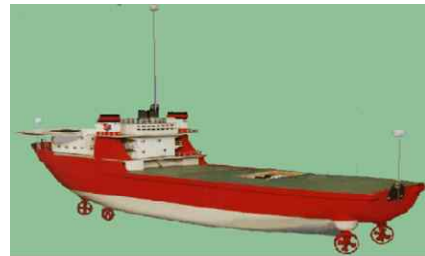
Fig. 3 Cybership I : scale 1:70 of a supply vessel
