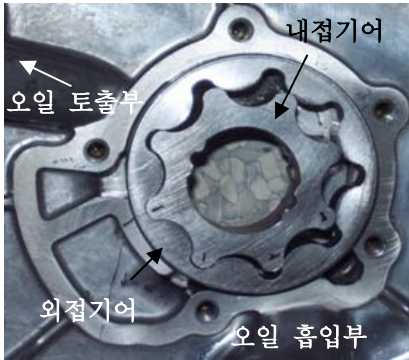
Fig 1. Gerotor Oil Pump
