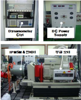
Figure 2 Experimental setup for the mechanical performance of an electric motor
