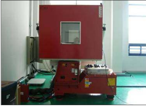
Fig. 2 The Electrical Vibration Tester
