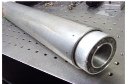
Fig.1 Dynamic damper into Drive Shaft
