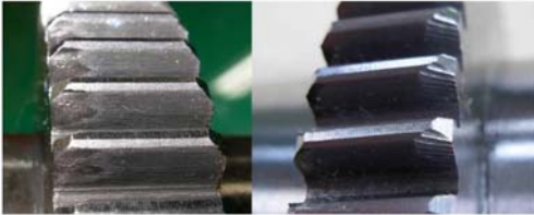
Fig. 2 Gear tooth weaned by misalignment
