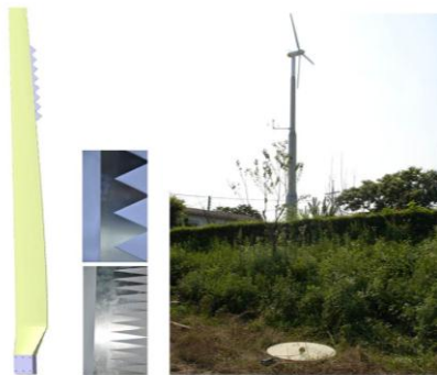
Fig. 8 The manufactured low noise serrated trailing edged blade and acoustic field test
