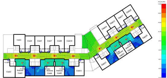
Figure 3 Improved design of the location of the alarm device in common corridor
