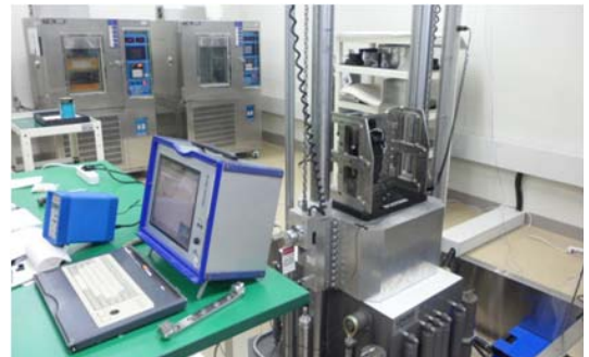
Fig. 9 Drop-table shock tester for scope shock test
