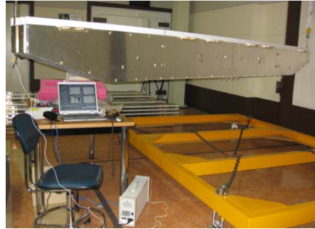
Fig. 7 Modal test of array-antenna pack-assy.
