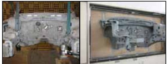
Fig. 2 Dash systems in experiment (left, suspended for sound radiation measurement; right, installed for TL buck test)
