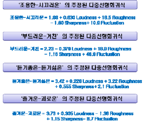
Fig. 2 Subjective response versus predicted results by multiple linear regression method for the data from SDM about feeling
