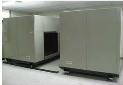
Fig. 1 Mini-chamber for measurement of sound transmission loss
