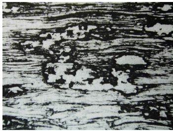
Fig. 2 Magnified photograph of worn surface of No.1 sintered brake pad
