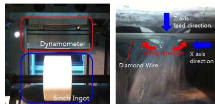
Fig. 2 Experiment setup & Slicing mechanism
