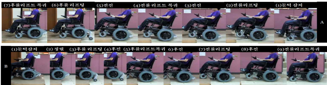
Fig. 5 Operation steps of the curb climbing wheelchair: Going up(A) and down(B) curbs
