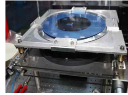
(b) Experimental setup for thin chip ejecting process
