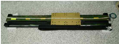
Fig. 4 Stage 2: Linear motor driven stage
