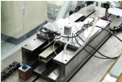
Fig. 5 Stage 3: Linear motor and air bearing stage
