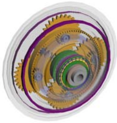
Fig. 2 MASTA-Model Planetary Gear Reducer
