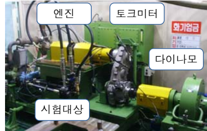
Fig. 4 Transfer Case Test Bed
