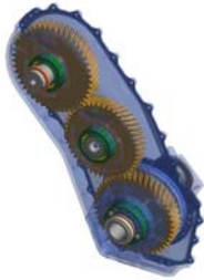
Fig. 2 MASTA-Model Transfer Case
