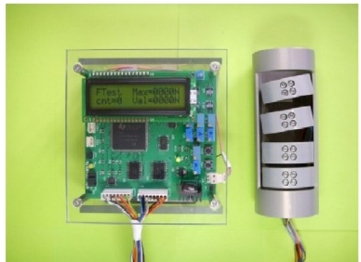
Fig. 2 Manufactured cylindrical-type finger force measuring system.
