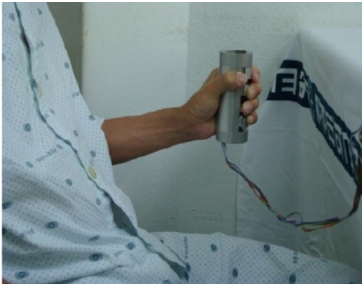
Fig. 3 Characteristics test of patients with finger paralysis using cylindrical-type finger force measuring system
