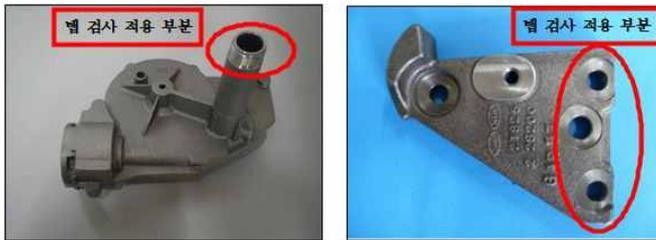
Fig. 1 Automotive parts with tapped
