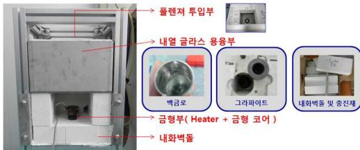
Fig. 1 Schematic of glass material dispenser system
