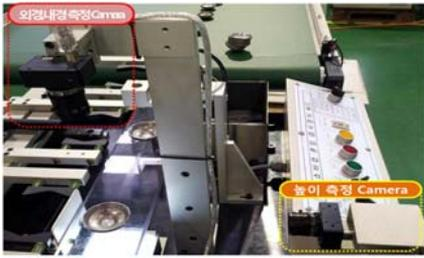
Fig. 4 Machine Vision System
