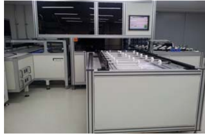
Fig. 6 Solar module Lay-up machine
