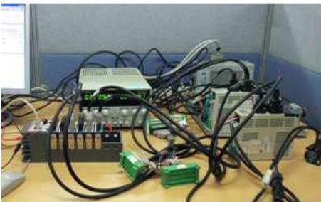
Fig. 4 Experimental setup for position and velocity control of winding and unwinding motor
