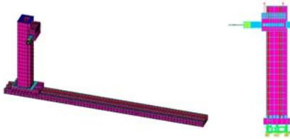
Fig. 3 Finite element model of FTBM
