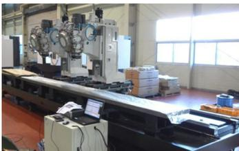
Fig. 5 Twin spindle line-center
