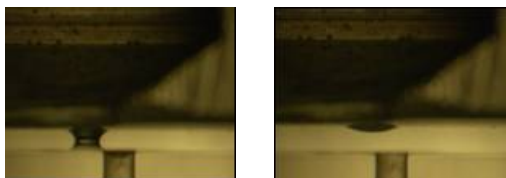
(a) Remained liquid bridge (d=0.6mm) (b) Ruptured liquid bridge (d=0.8mm)
