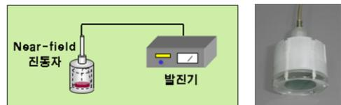
Fig. 1 (a) System configuration of the near-field megasonic waveguide with the electric generator and (b) the fabricated waveguide.
