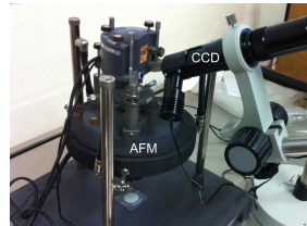
Fig. 1 AFM and CCD system for nano electrochemical machining in a electrolyte droplet
