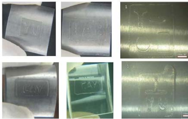
Fig. 3 Fabricated SU-8 rapid mask
