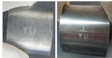
Fig.6 Carved shapes onto 3D non-planar wafer
