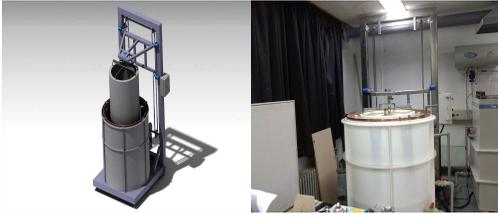
Fig. 3 Equipment of the electroforming system
