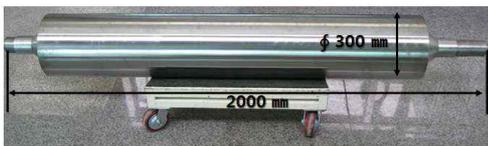
Fig. 1 Nickel plated roll molds<sup>3</sup>
