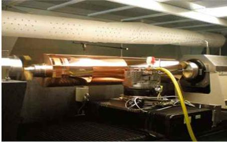
Fig. 2 Ultra Precision Drum Lathes
