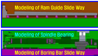
Fig. 3 Spring modeling of spindle bearing, boring bar slide way and ram slide way
