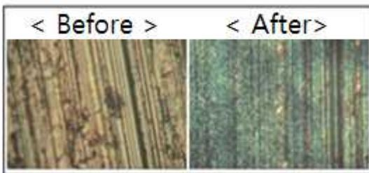
Fig. 4 Optical microscope images of the surface after e-beam irradiations
