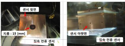
Fig. 2 Sensor for condenser current
