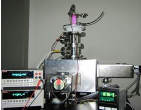
Fig. 2 Photograph of finishing process system using AC plasma.
