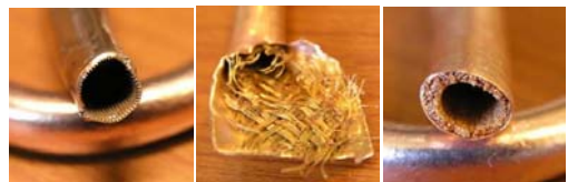
(a) Grooved Wick (b) Metal Mesh Wick (c) Metal Sintered Powder Wick
