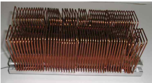
Fig. 1 Cooling module using oscillating heat pipe
