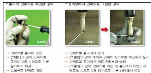
Fig. 2 Locking and exchange of insert tip
