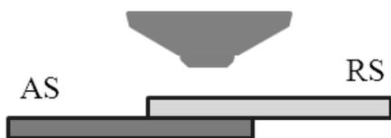
Fig. 1 Schematic illustration of FSW tool & specimen position.
