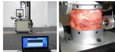
Fig 2. L4-L5 specimen for nucleotomy & mounted with spine tester. the axial force was applied by loading apparatus.
