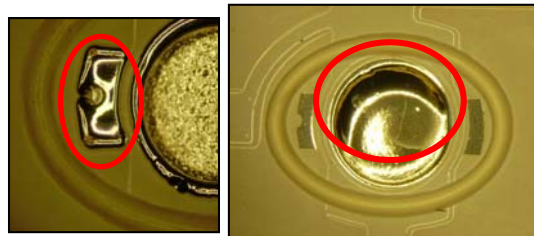
Fig. 3 Defective Phenomenon of plating
