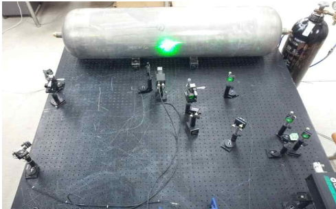
Fig. 2 Photography of Out-of-Plane ESPI Setting
