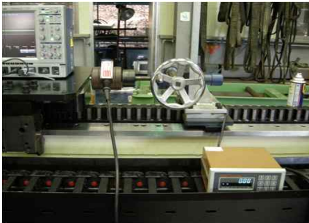
Fig. 4 Picture of liner motor thrust test system
