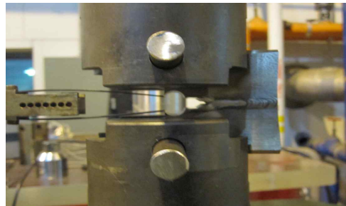
Fig. 1 Fracture Toughness Testing for Weld Curved CT specimen
