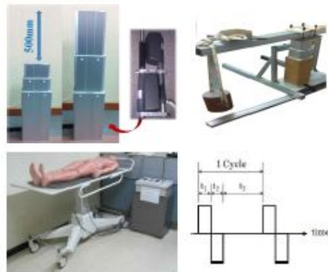
Fig. 3 Static and Dynamic Loading Tests for 3-step Column Lifting Module
