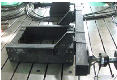
Fig. 4 Load testing system of rear protector
